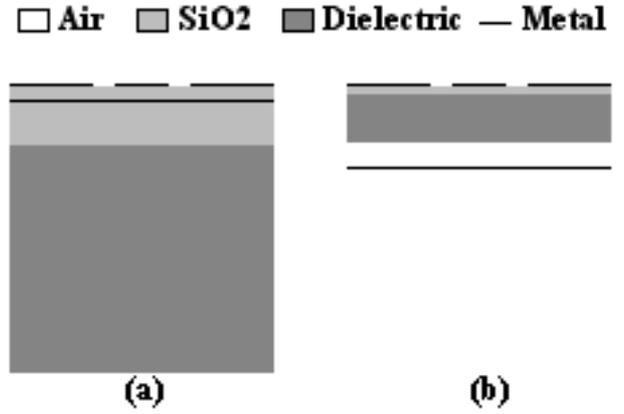
Fig.5: Area in which a ground plane can be. (a)As a shield on the second metal layer or (b)outside of the die
