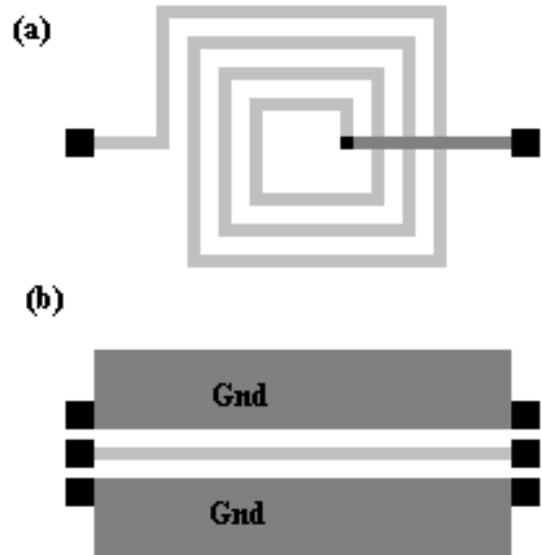
Fig.1: Inductors : (a)classical square spiral and (b)CPW
