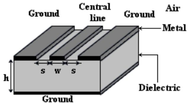
Fig.2: Coplanar waveguide (CPW)
