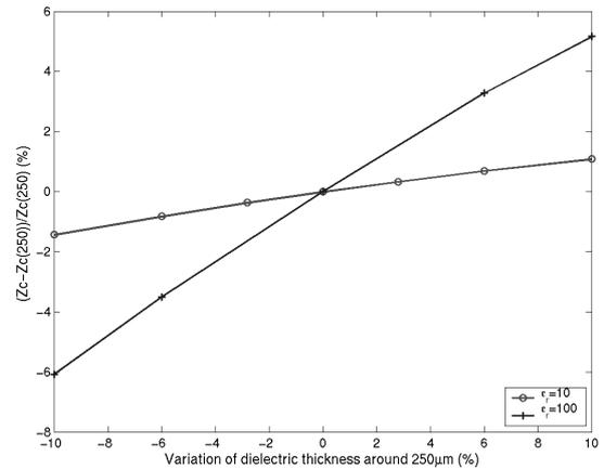
Fig.8: Variation of  $Z_c$  with the variation of the ground plane position just under the chip
