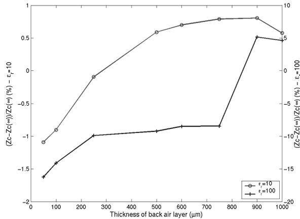
Fig.7: Variation of  $Z_c$  with the air substrate layer thickness
